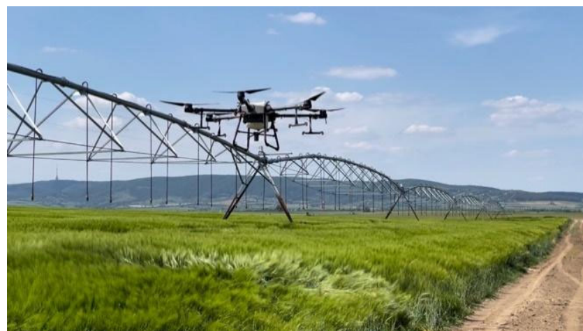
Figure 2. Spraying barley crops in the zone of the irrigation system, which is inaccessible to tractor sprayers.
