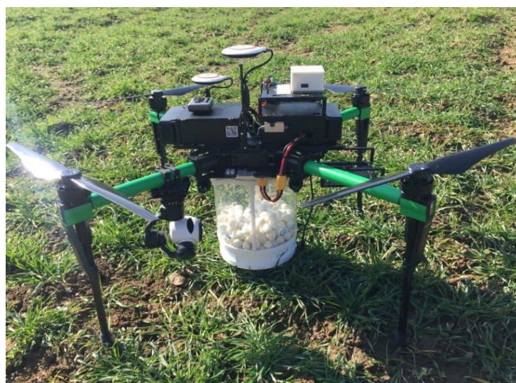
Figure 3. Drone DJI Matrice 100 for Trichogramma application (taken from https://www.drone-store.it/ ; accessed on 1 July 2023).
