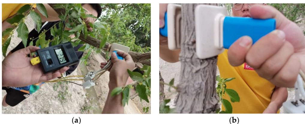
**Figure 2.** Experimental methods for heating jujube bark: (a) experimental method for initial heat transfer model; (b) heating experimental method for final heat transfer model with the function of the bark thickness prediction.
