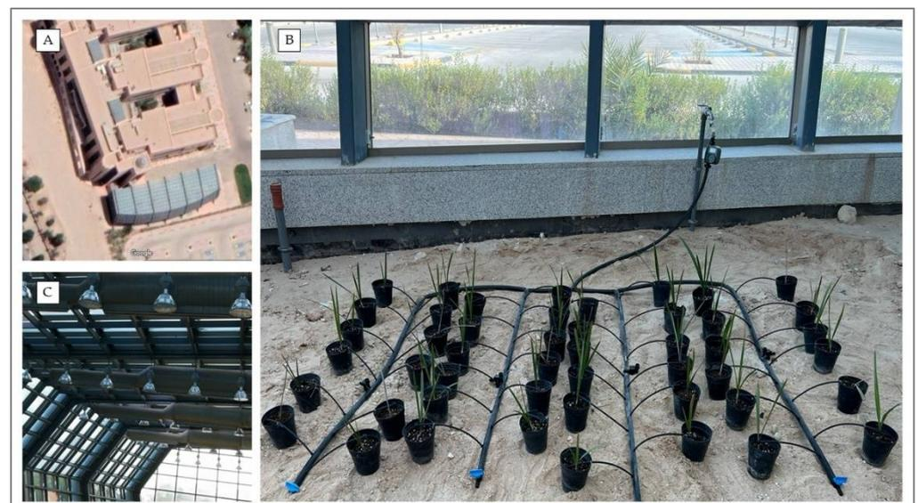
**Figure 7.** The experimental setup of TCPs for acclimatization in the TGAS. (A) Screenshot from Google of the glasshouse site, (B) The experimental setup, (C) Air conditioning and lighting systems in the glasshouse.
