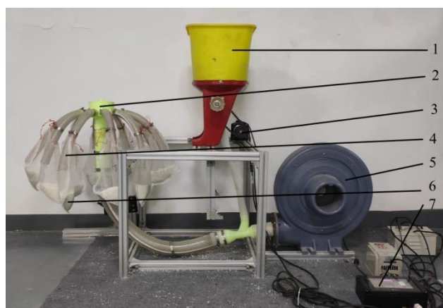
Figure 12. Pneumatic fertilizer discharge device bench. (1) fertilizer box, (2) distributor, (3) stepper motor, (4) fertilizer discharge tube, (5) centrifugal fan, (6) yarn bag, (7) test bench controller.
