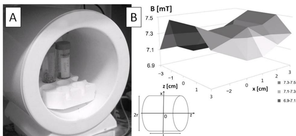
**Figure 1.** Exposure system. (A) Plant material in the coil. (B) The average magnetic flux density distribution inside the solenoid along the Z and X axes. Inset shows the coordinate system.  $2r$ —diameter of the solenoid,  $B$ —magnetic flux density vector,  $l$ —coil length.
