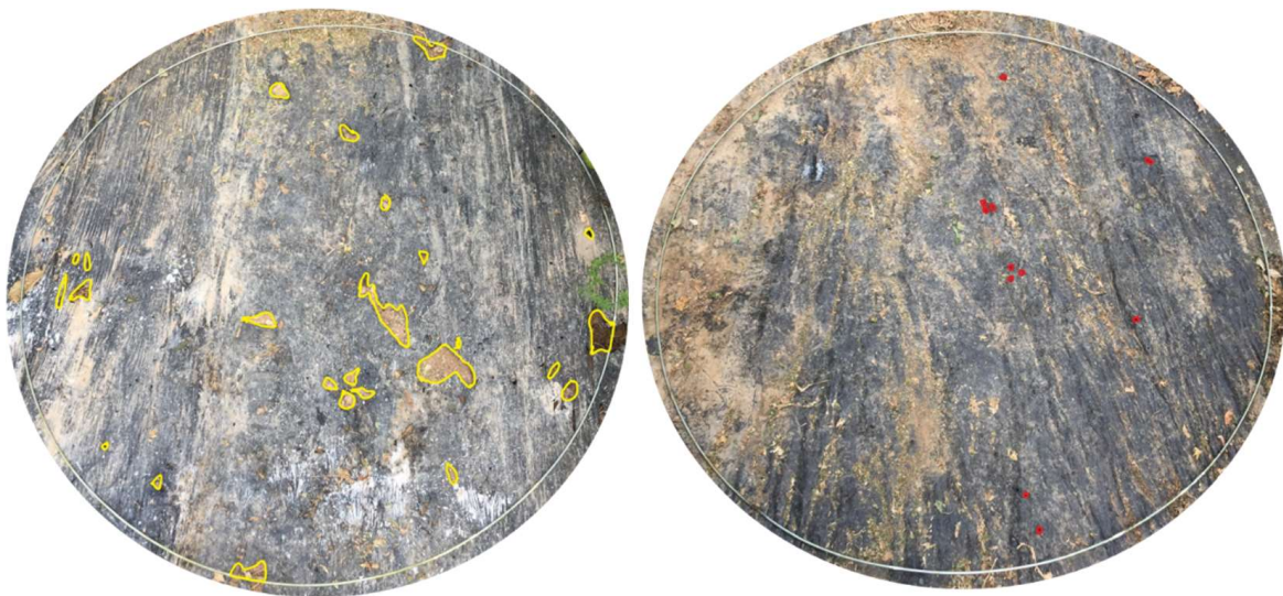
Figure 8. Visual deterioration of biodegradable biopolymer ((left); deteriorated area in yellow color) and polyethylene ((right); deteriorated area in red color) plastic mulches at the end of the crop season in Year 2 (195 days after planting). Surfaces occupied by the ring (1 m 2 ) were processed with software to obtain the deteriorated area (perforations and/or breaks).
