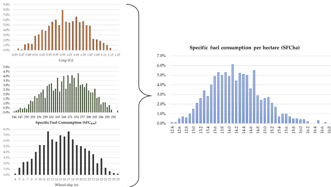
**Figure 2.** Percentage frequency distributions of the three random input variables ( $G$ ,  $SFC_{kW}$ , and  $s$ ) and the output ( $SFC_{ha}$ ) of the Monte Carlo Simulation.
