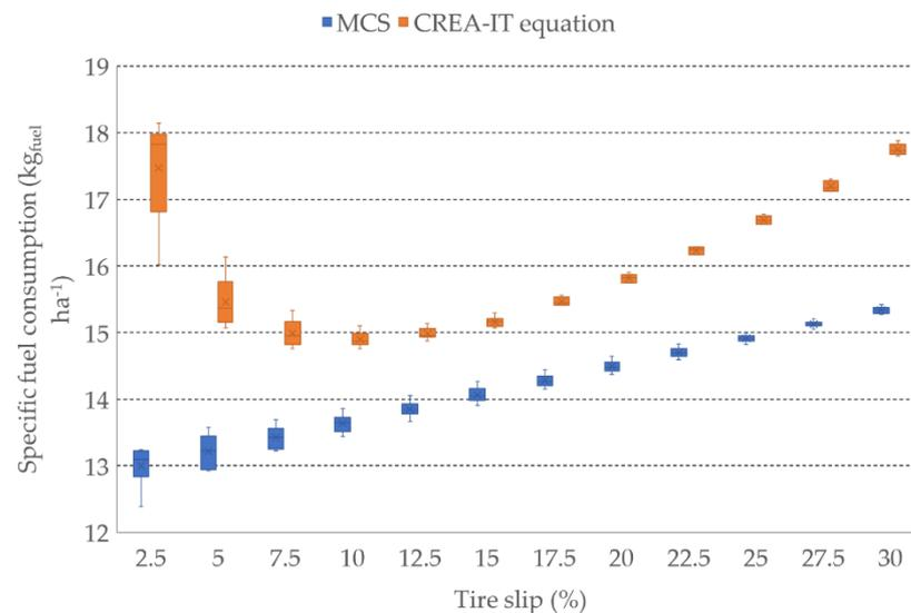
**Figure 6.** Comparison of the specific fuel consumptions ( $\text{kg}_{\text{fuel}} \text{ha}^{-1}$ ) resulting from the Monte Carlo algorithm and the CREA-IT output.
