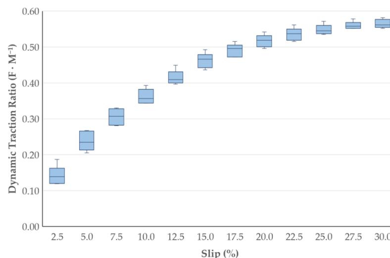
**Figure 4.** Boxplots representing the dynamic traction ratio during tests carried out at various levels of slip (highest and lowest data values, median, first and third quartiles).
