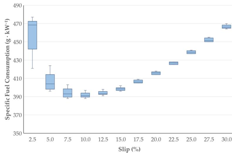
**Figure 5.** Boxplots representing the specific fuel consumption of the power at the drawbar during the tests carried out at various levels of slip (highest and lowest data values, median, first and third quartiles).
