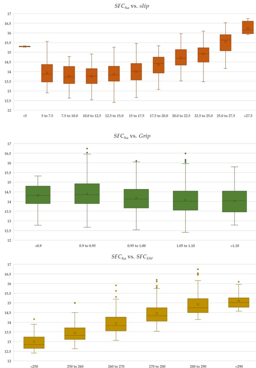
**Figure 3.** Boxplots (highest and lowest data values, median, first and third quartiles) representing the distributions of the model output ( $SFC_{ha}$ ) vs. the simulated wheel slip, tire grip, and the specific fuel consumption of the engine ( $SFC_{kW}$ ). Dots “.” represent outliers.
