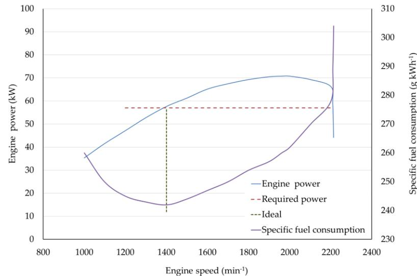
**Figure 1.** Example of the shape of the maximum  $P_{PTO}$  and the relative  $SFC_{kW}$  of a 71 kW tractor. A representation of the required power and the “ideal” working point in terms of efficiency is provided (i.e., 57 kW at 1400  $\text{min}^{-1}$ ).
