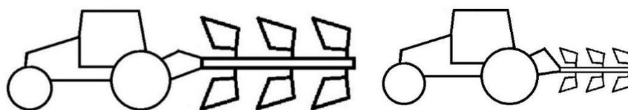
**Figure 7.** Examples of incorrect coupling of the implement and the tractor size. The mismatch results in the inability to manage the operational parameters efficiently.
