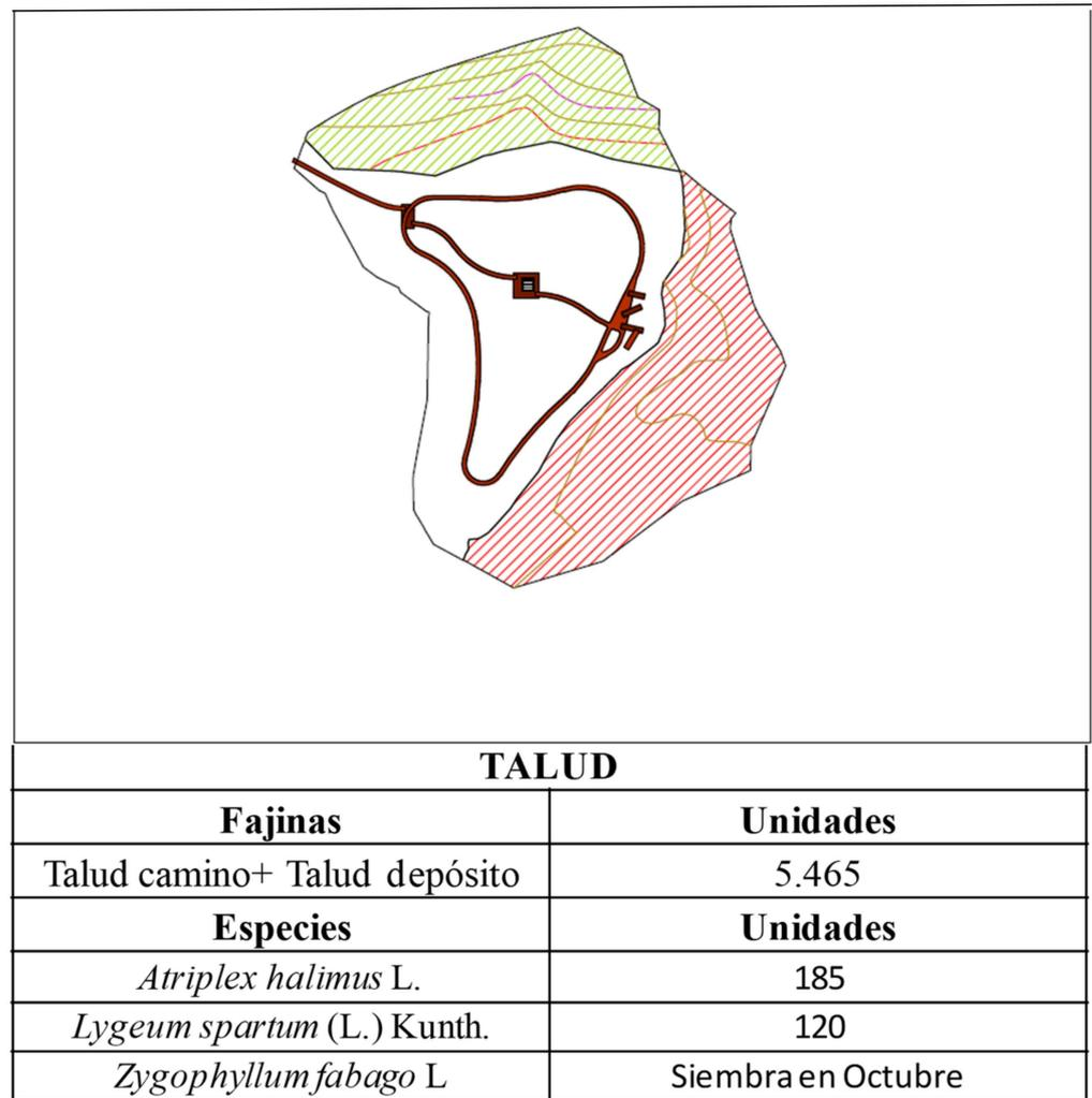
Figure A10. Planting plan for the stabilization of slopes of Case Study 1.
