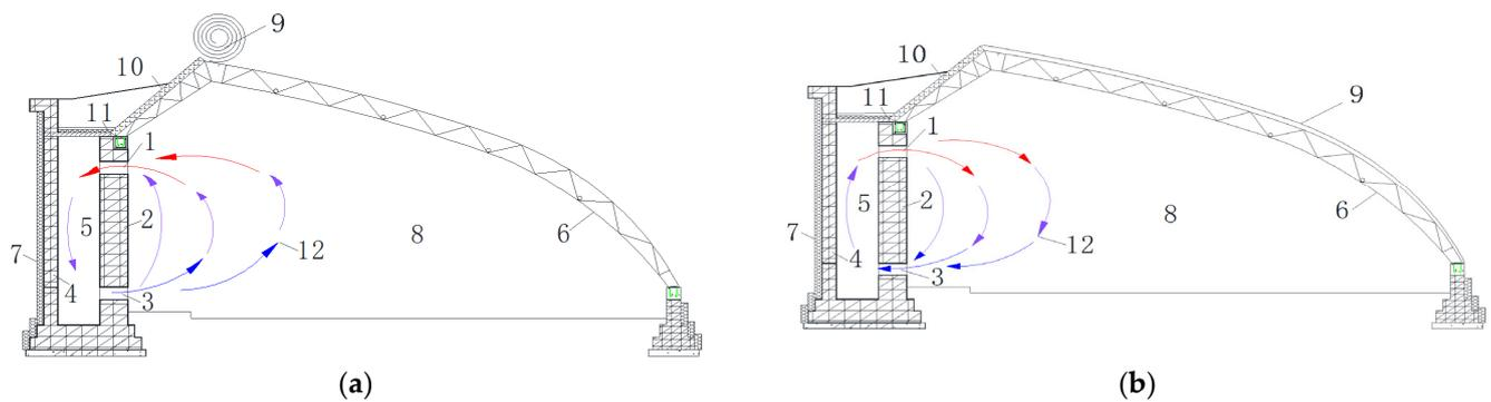
**Figure 2.** Circulation direction of natural convection: (a) circulation direction during the day; and (b) circulation direction at night. (1) Upper vent, (2) inner layer of north wall, (3) lower vents, (4) outer layer of north wall, (5) hollow layer, (6) gable south roof frame, (7) insulation layer, (8) cultivation space, (9) thermal blanket, (10) north rear roof, (11) insulation layer, and (12) direction of airflow (Red indicates hot air and blue indicates cold air).
