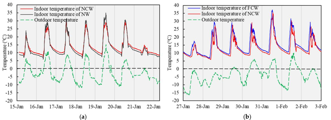
**Figure 5.** Comparison of indoor and outdoor temperatures under different conditions: (a) NCW and NW; and (b) NCW and FCW.
