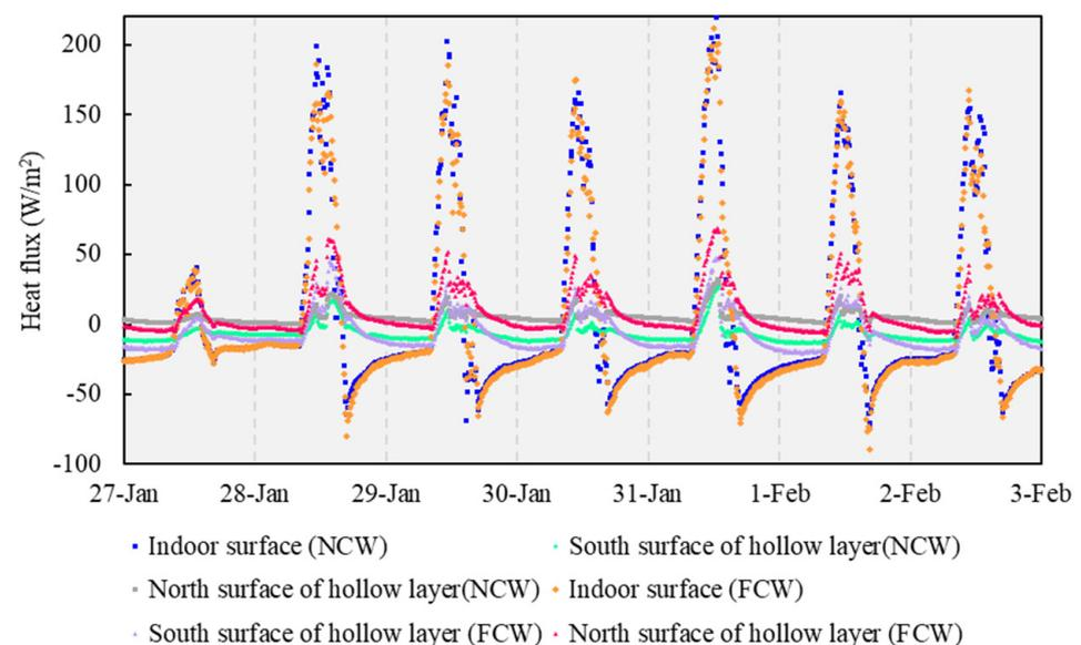
**Figure 8.** Heat flux of different surfaces of the NCW and FCW.
