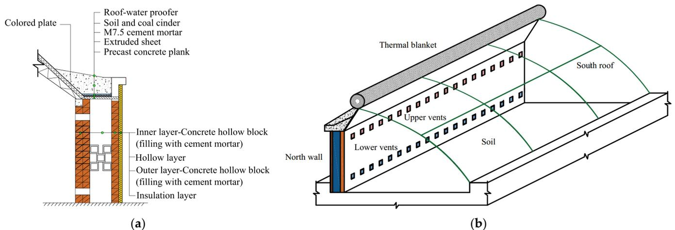
**Figure 1.** Structure of the air convection heat storage north wall: (a) Schematic of the air convection north wall with a hollow structure; and (b) schematic of the indoor surface with vents.
