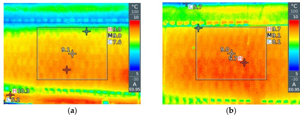
**Figure 10.** Wall surface temperatures of the FCW and NCW at 06:00 (January 24, 2018): (a) FCW; and (b) NCW.
