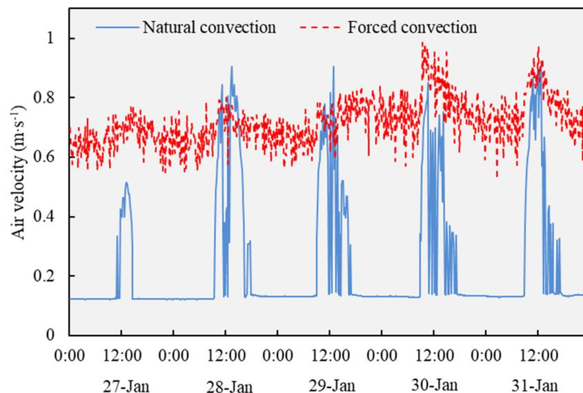
**Figure 11.** Air velocity of the vents under natural convection and forced convection.
