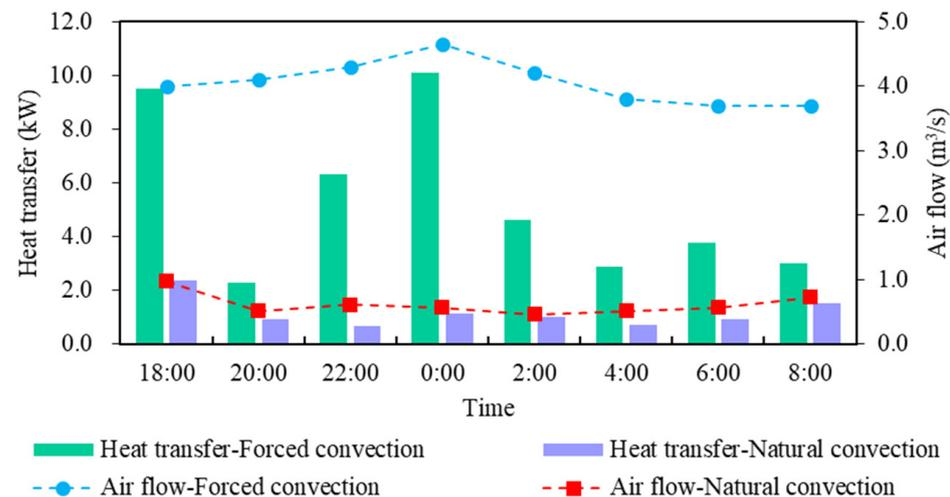
**Figure 13.** Airflow and heat transfer of forced and natural convection at night (January 23).
