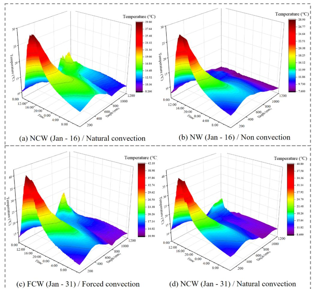
**Figure 6.** Internal temperature distribution of the wall with blocked internal convection (NW), wall with natural internal convection (NCW), and wall with forced internal convection (FCW) on a sunny day.
