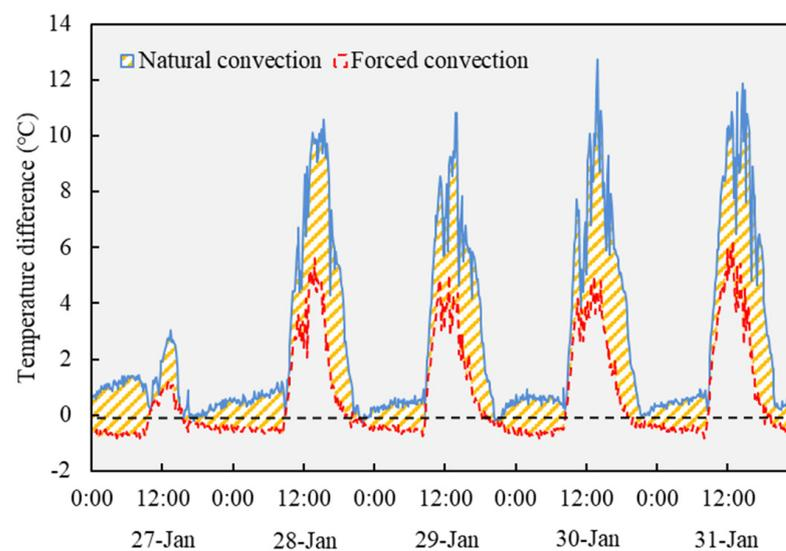
**Figure 12.** Temperature difference between the upper and lower vents of the NCW and FCW.
