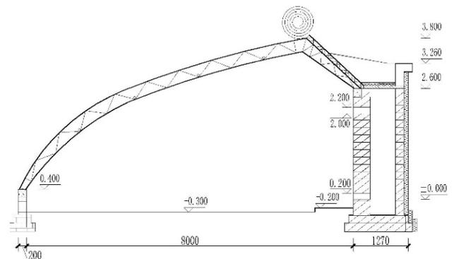
**Figure 3.** Field and structure of the experimental Chinese solar greenhouse. Note: The units of height and span are meter (m) and millimeter (mm), respectively.
