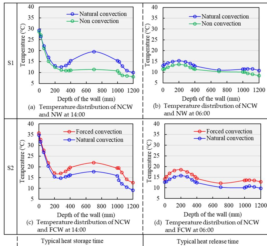
**Figure 7.** Temperature distribution in the wall at the typical thermal storage time (14:00) and release time (06:00) on a sunny day. Note: Wall depth was calculated in the indoor direction to the outdoor direction.
