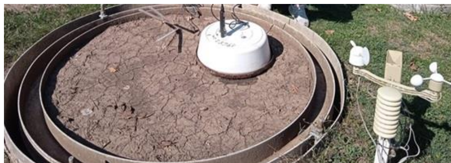
Figure 3. The setup of the frame–bowl method to measure the CO 2 efflux from undisturbed soil under field conditions.
