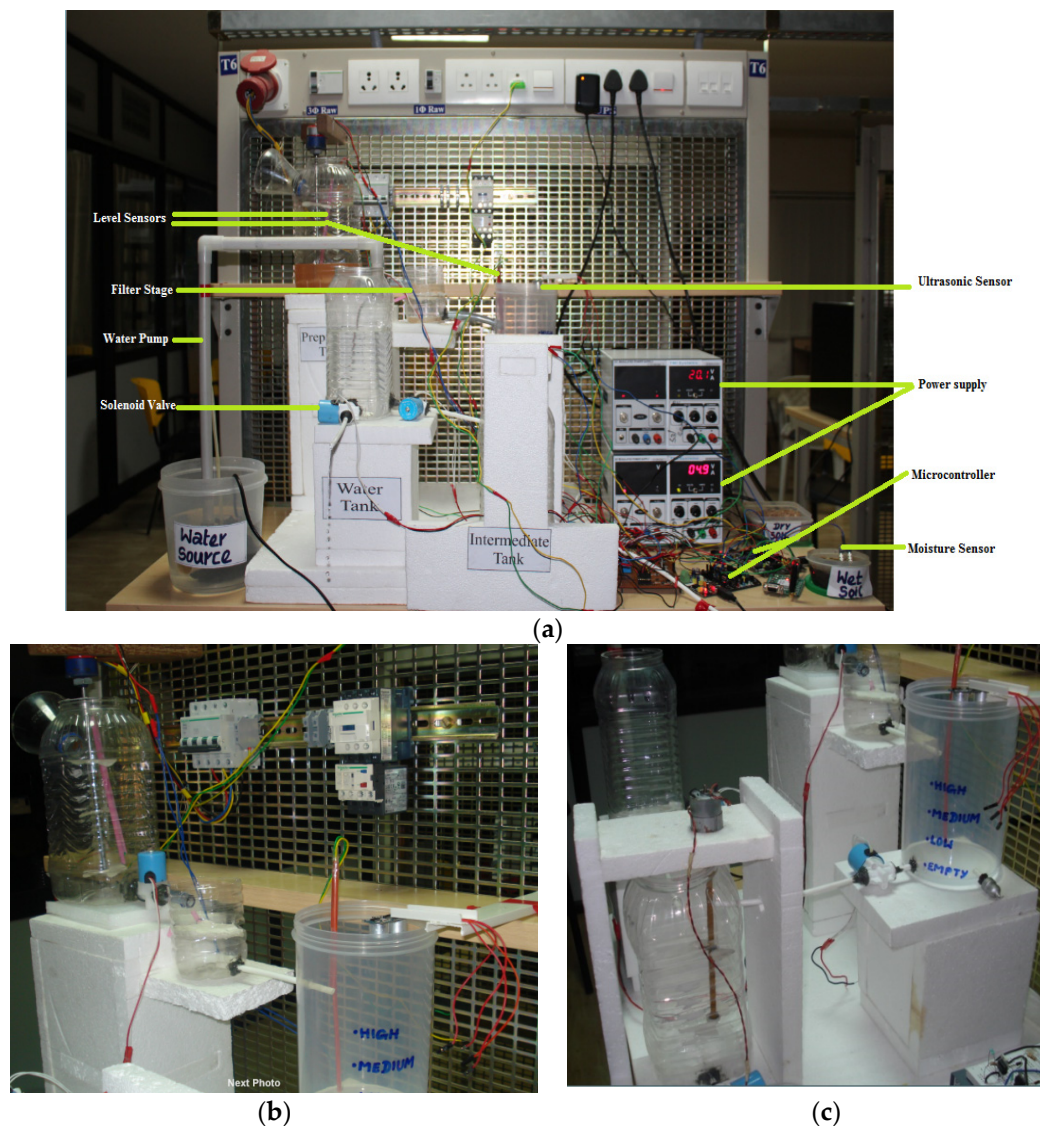
Figure 4. (a) Hardware setup of the proposed pilot scale model, (b) implementation of the preparation module, and (c) implementation of the irrigation module.
