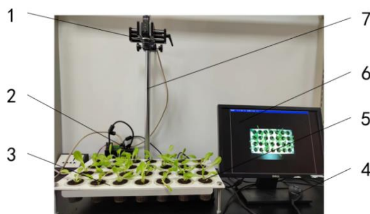
Figure 9. Test equipment: 1. Camera. 2. Controller. 3. Seedling tray. 4. Operating handle. 5. Transplanting cup. 6. Monitor. 7. Stand.
