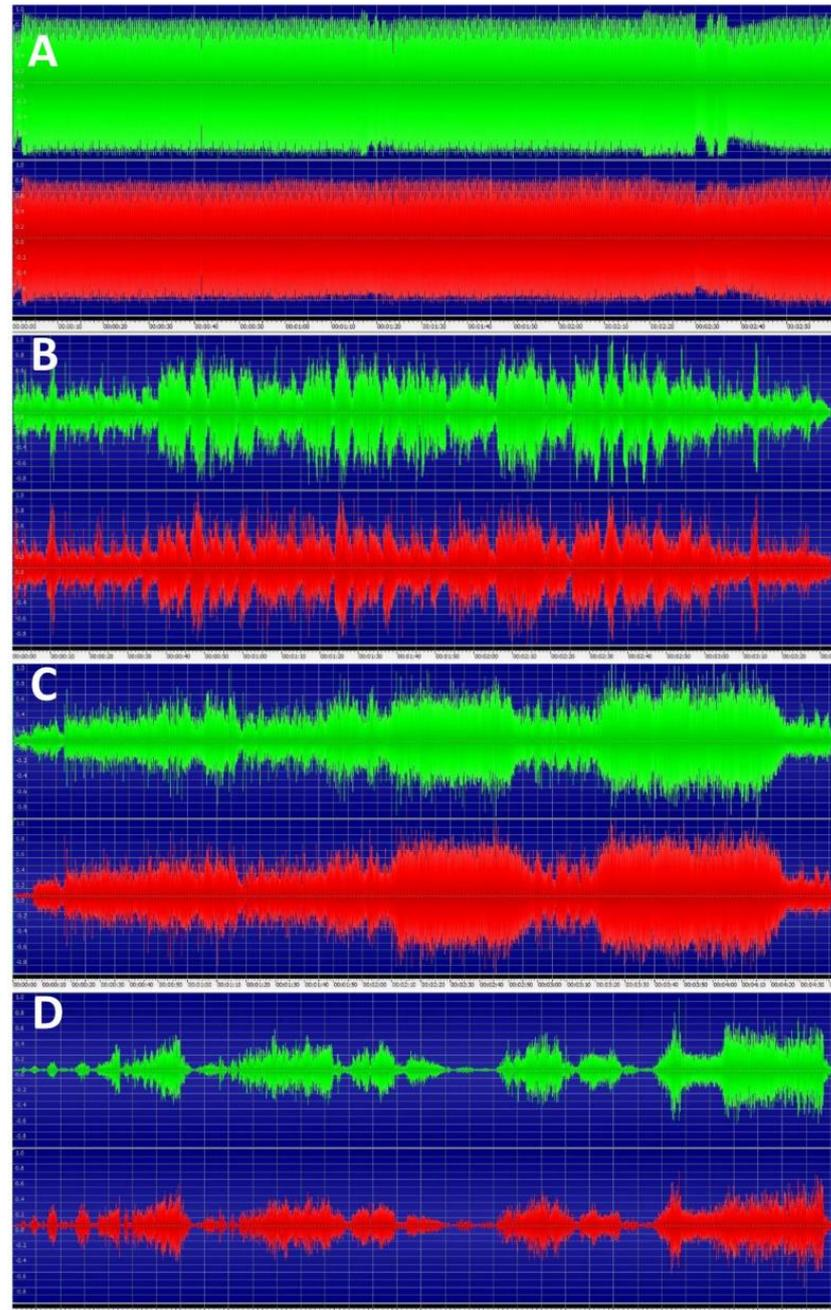
**Figure 2.** Acoustic characteristic diagram (A: PAFT; B: EM; C: RM; D: CM); The sampling rate of the frequency spectrum analysis software GoldWave was 44,100 Hz for the MPEG format of the sound samples, and the green and red waveforms represent the left and right channels, respectively.
