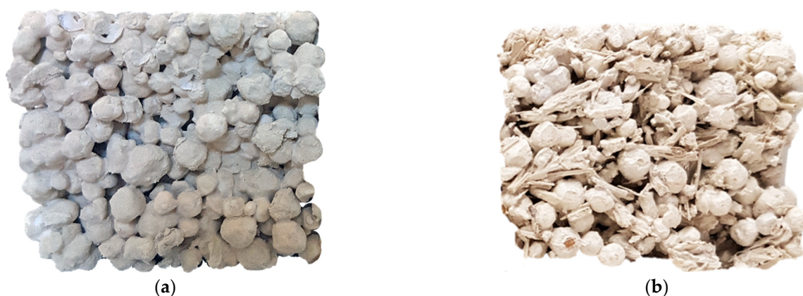
Figure 8. Samples of bonded leveling compound (a) CP 0 in Binder 1 ; (b) CP 30 in Binder 2 .
