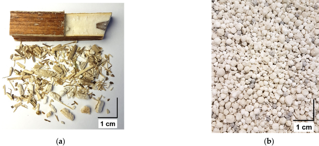
Figure 5. Lightweight aggregate examples (a) Cup plant stem and milled sieve fraction; (b) Expanded polystyrene aggregates (sieve fraction: 1–6 mm) [Scalebar = 1 cm].
