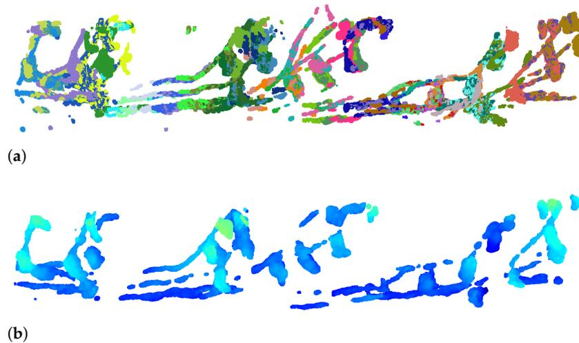
**Figure 7.** Images of a point cloud using 50 successive images of the greenhouse row before and after applying outlier removal. (a) Point cloud created using 50 successive images. The points from each image are displayed in a random colour. (b) Point cloud after outlier removal. Points are colorized based on distance from the camera, where blue-green points are closest to the camera (approximately 0.3 m), while dark blue points are farthest away (approximately 0.7 m).
