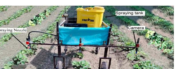
Figure 6. Schematic diagram of variable rate sprayer in field evaluation experiment.
