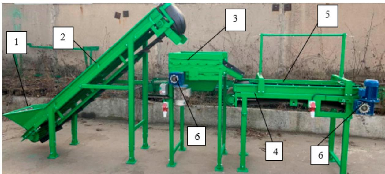
**Figure 3.** Photograph of a machine for the post-harvest processing of potato tubers with an automated sorting system: 1—receiving hopper; 2—transfer conveyor; 3—spiral heap cleaner; 4—sorting table; 5—conveyor belts; 6—electric motors.
