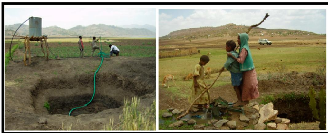
**Figure 6.** Groundwater abstraction using the treadle pump.
