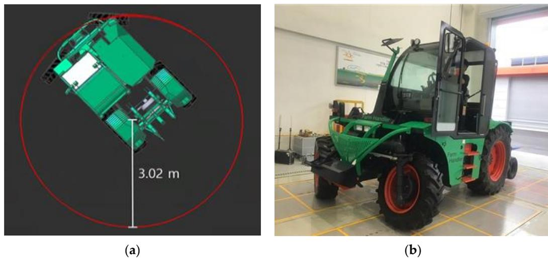
**Figure 5.** Minimum turning radius from the simulation and certified performance test: (a) simulation; and (b) measurement.
