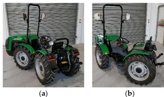
**Figure 2.** Articulated tractor: (a) articulation to the left; (b) articulation to the right.
