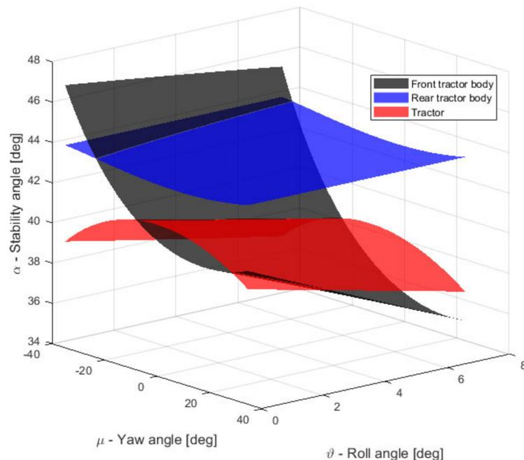
**Figure 7.** The stability angles of the separate bodies and the whole tractor vs. Yaw angle and Roll angle. Front body (black surface), the rear body (blue surface) and the whole tractor (red surface).
