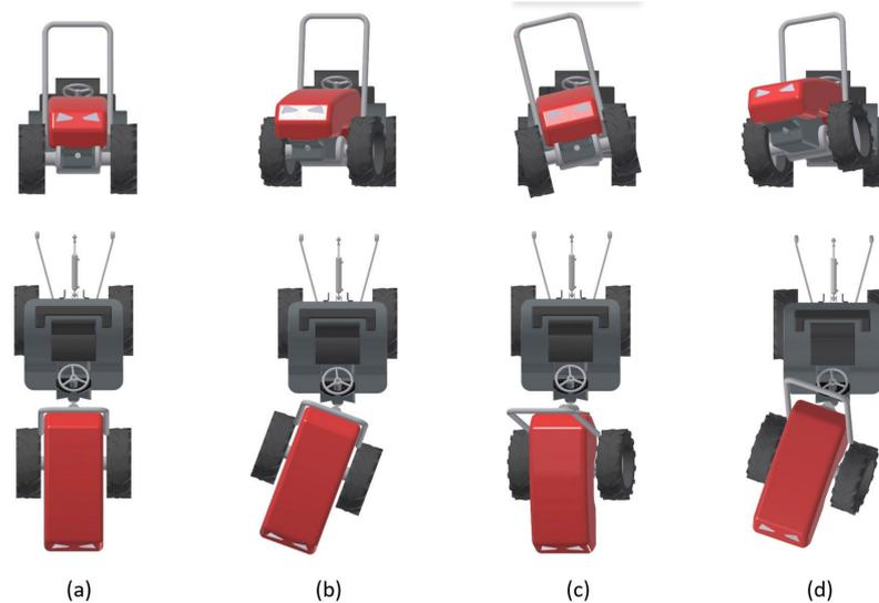
**Figure 4.** The configurations of the compact articulated chassis tractor: (a) Straight; (b) Yaw angle; (c) Roll angle; (d) Yaw and Roll angles.
