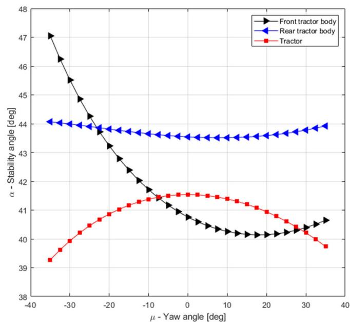
**Figure 9.** Tractor in the articulated configuration: tractor stability angles vs. Yaw angle. Front tractor body (black line), rear tractor body (blue line) and whole tractor (red line).
