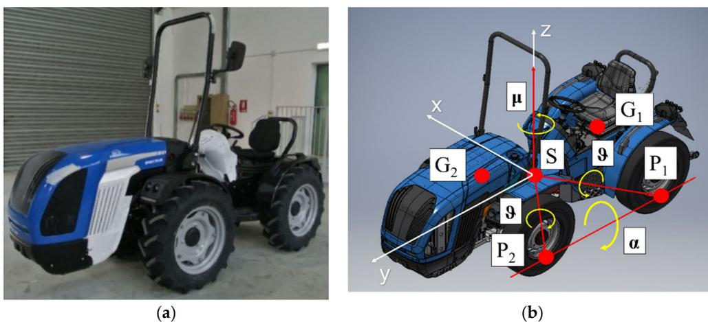
**Figure 3.** Compact articulated tractor: (a) Actual tractor in the straight configuration; (b) Graphical representation of the tractor parameters assumed in modelling:  $P_1$ ,  $P_2$ ,  $G_1$ ,  $G_2$  and  $S$  are the five characteristics points defined in the modeling approach related to the geometrical tractor configuration,  $\mu$  is the yaw angle,  $\theta$  is the roll angle and,  $\alpha$  is the tractor stability angle.
