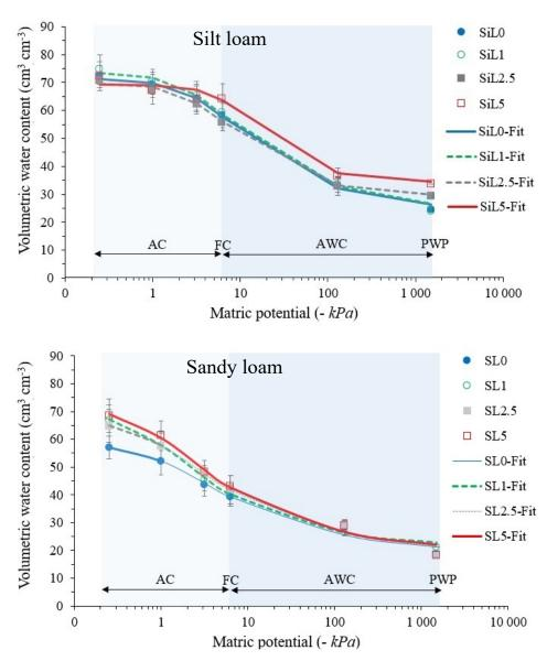
**Figure 5.** Water retention curve for the silt loam (SiL) and sandy loam (SL) materials and their mixtures with 1, 2.5, and 5 wt.% bamboo biochar. Observed data were fitted with the van Genuchten–Mualem model by means of the RETC software [46].
