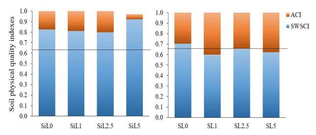
**Figure 6.** Soil Water Storage Index (SWSCI) and Air Capacity Index (ACI) for the silt loam (SiL) and sandy loam (SL) mixtures. The horizontal continuous line represents limit index values suggested by Reynolds et al. [41].
