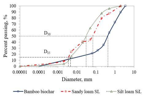
**Figure 3.** Particle size distribution of the bamboo biochar (squares and continuous blue line), and the soil materials: sandy loam (circles with dashed red line) and silt loam (triangles with dotted green line).
