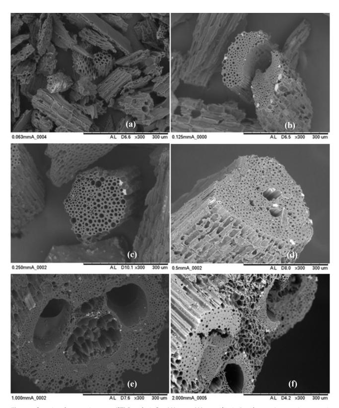
Figure 4. Scanning electron microscope (SEM) analysis (bar 300  $\mu$ m imes 300 magnification) to characterize porosity composition of the different bamboo biochar particle sizes of (a) 0.063 mm, (b) 0.125 mm, (c) 0.250 mm, (d) 0.500 mm, (e) 1.0 mm, and (f) >2 mm.
