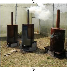
**Figure 1.** Carbonization kilns designed at the Costa Rica Institute of Technology for biochar production: (a) pyrolysis chambers of three kilns (behind) and halved bamboo stems (at left); (b) reactor during production.
