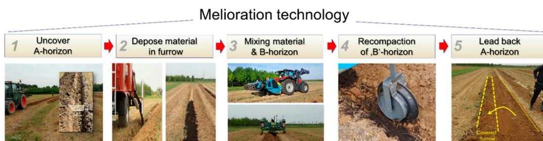
**Figure 2.** Phases of the Soil<sup>3</sup> melioration process and selected photos of the technology from the preliminary tests for tool selection and design.
