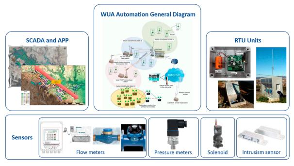
Figure 2. Scheme of automation system in Pliego water users association (WUA).
