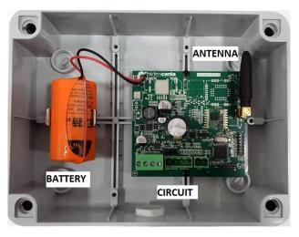
Figure 6. Smart Agri equipment and components (single user in a micro-plot).
