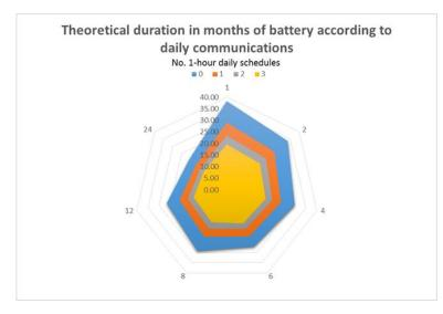
Figure 9. Battery duration according to number of communications.
