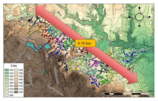
Figure 5. Distribution of hydrants for remote control in Pliego WUA.
