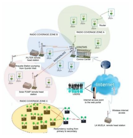
Figure 12. Integration scheme of different systems.
