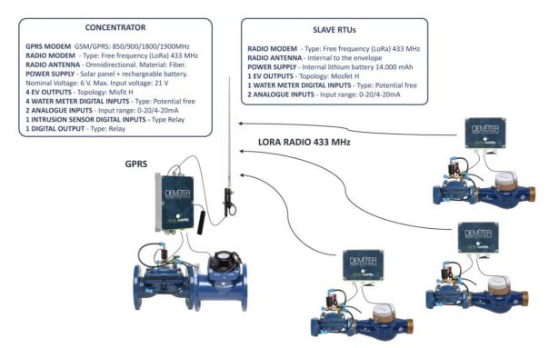
Figure 3. Descriptions of sensors in Pliego WUA.
