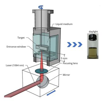
**Figure 1.** The experimental setup used for carbon nanoparticle (CNP) generation through the pulsed laser ablation in liquid (PLAL) method. The inset digital image shows the daylight appearance of the obtained CNP suspension in ethanol.
