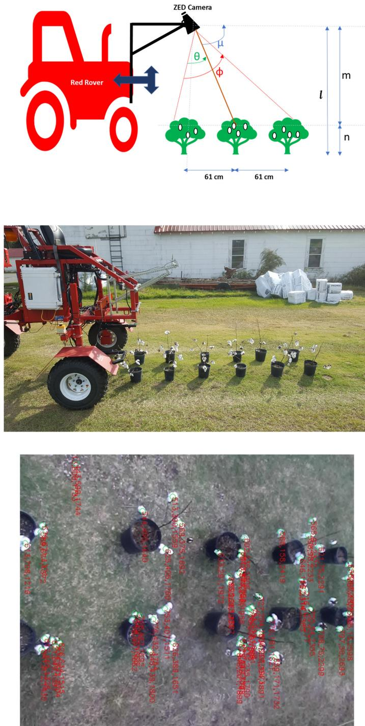
Figure 9. Context diagram that shows cotton boll position measurements.
