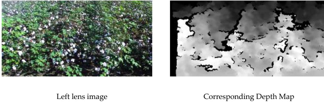
**Figure 11.** Collected RGB image and corresponding depth map for cotton row detection (0–255, 8-bit greyscale image).
