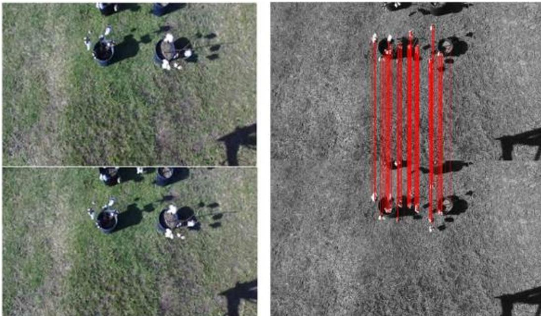
**Figure 8.** Two consecutive images collected from the ZED camera and the moving rover (left images) and matching features obtained using the oriented FAST and rotated BRIEF (ORB) algorithm and the homograph random sample consensus (RANSAC) algorithm (right image).
