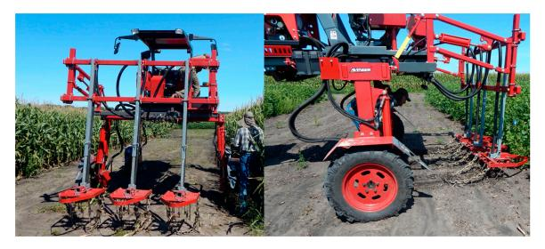
**Figure 1.** Modified Avenger high-clearance tractor outfitted with a Gandy Co. Orbit Air Seeder. Drop stanchions support cover crop seed delivery housing and soil incorporation units. Photo credit: Eric Ristau.
