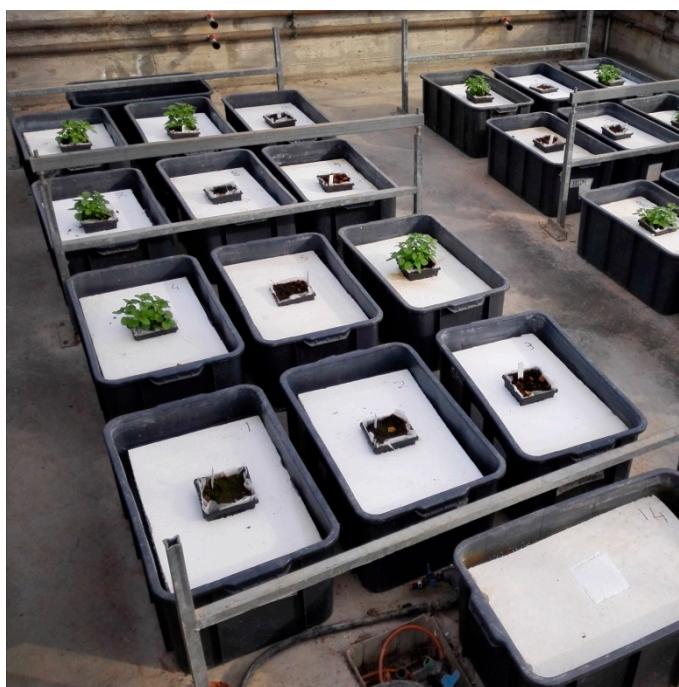
Figure 1. Photograph of the experimental site showing the plastic crate boxes filled with the polystyrene panels floating on the water and bearing the net pots containing the substrates and, according to the experimental design, Mentha aquatica L. plants. At the bottom right of the picture, a crate box without pot and plant was used to evaluate water losses by evaporation.
