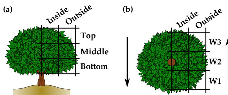
**Figure 2.** Sections of the canopy considered for average leaf area density ( $LAD_t$ ) estimation. (a) Side view across the row and (b) top view of a standard citrus tree. Arrows indicate the forward direction of the sprayer.
