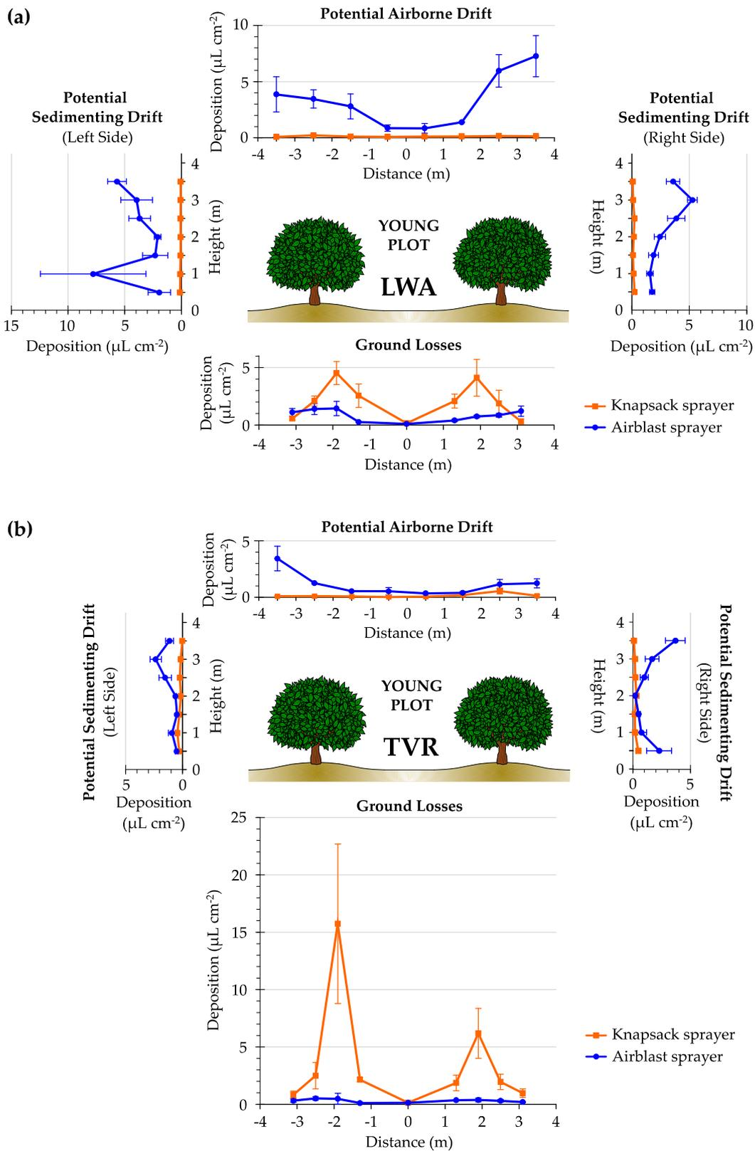
**Figure A4.** Off-target losses (mean (s.e.),  $\mu\text{L cm}^{-2}$ ) with the knapsack and the air-blast sprayer in the young plot and with dose expression using (a) LWA and (b) TRV.
