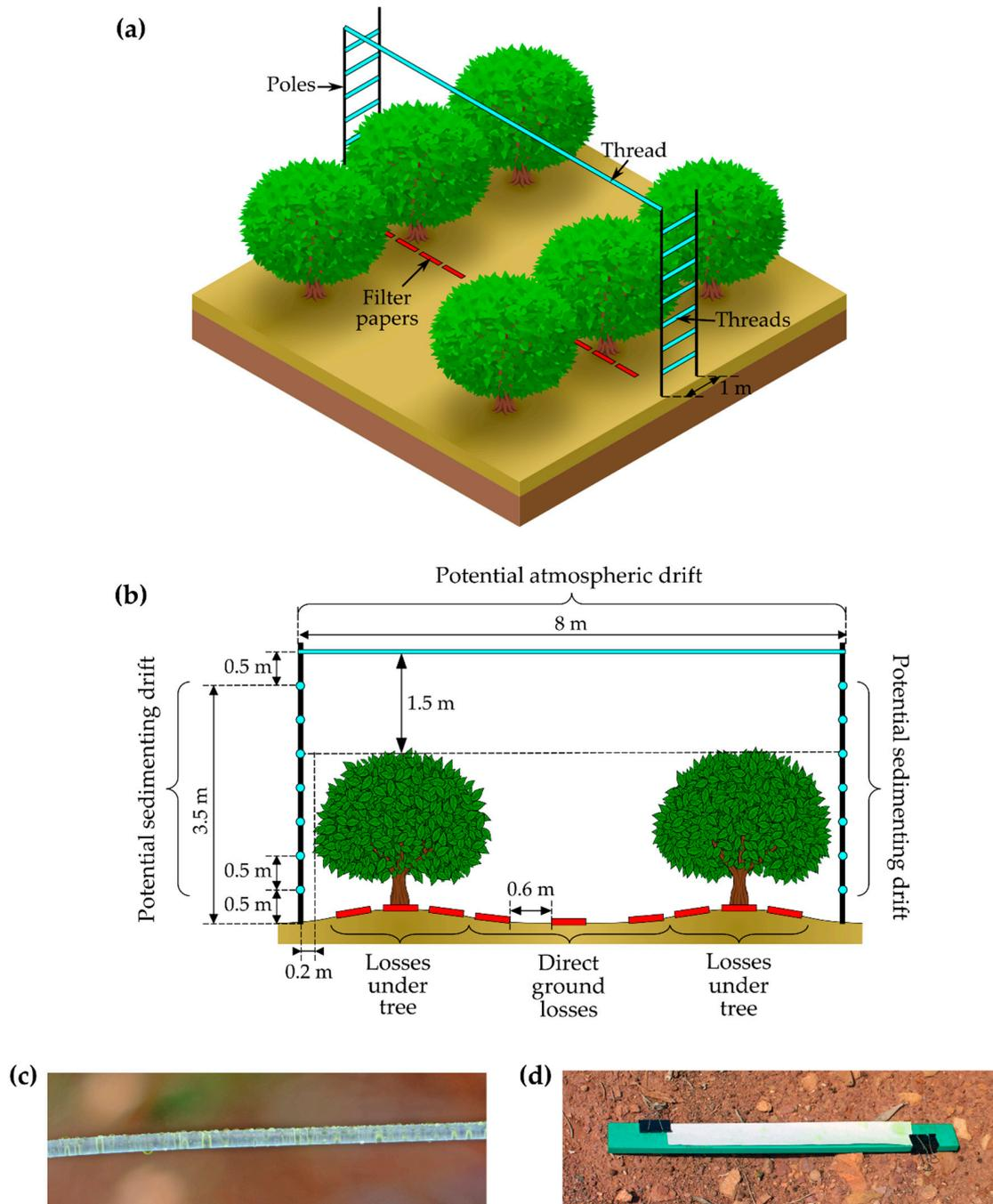
**Figure 7.** Collectors of off-target losses: (a) perspective and (b) side view across the row of the young plot with the structure provided by the collectors to estimate the potential drift and losses to the ground. The potential-drift-collecting threads are shown in light blue, and the ground-loss-collecting filter papers are shown in red. Collectors used: (c) nylon thread to estimate the potential drift and (d) filter paper to estimate ground losses.
