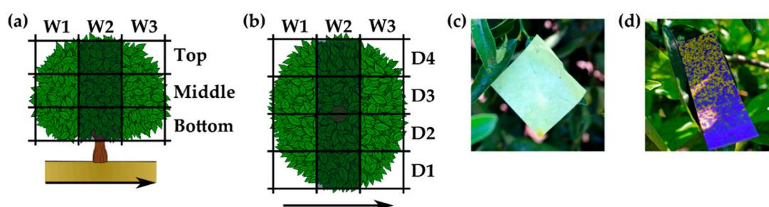
**Figure 6.** Quadrants of the canopy where the collectors were placed (shaded): (a) side view along the row and (b) top view. The arrows indicate the direction of the sprayer. Collectors used: (c) filter paper to estimate leaf deposition and (d) water-sensitive paper (WSP) to estimate spray coverage.
