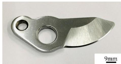
Figure 1. SK-5 High-carbon steel pruner.
