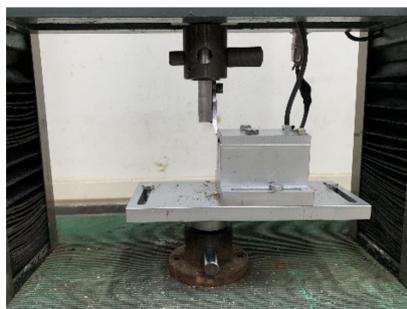
Figure 4. Shearing platform of universal tester.
