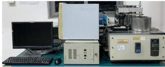
Figure 6. HT-500 high temperature friction and wear tester.
