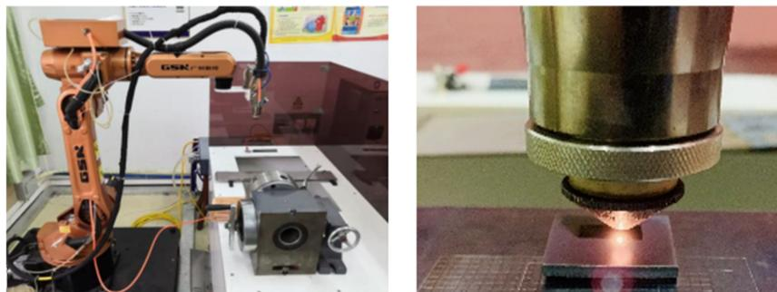
Figure 2. Laser manufacturing workstation of industrial robot.
