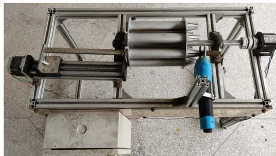
Figure 8. Self-made electric pruning deck.
