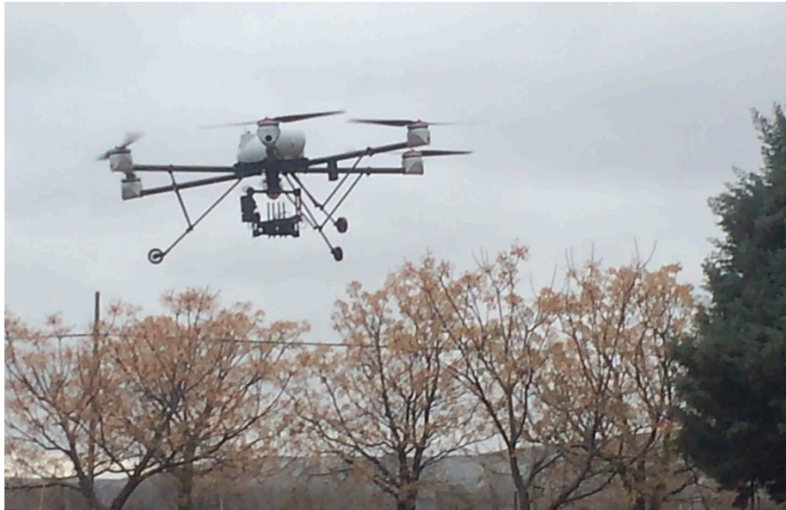
Figure 10. Hexrotor (AirRobot AR-200) carrying a vision camera for remote detection of weeds.
