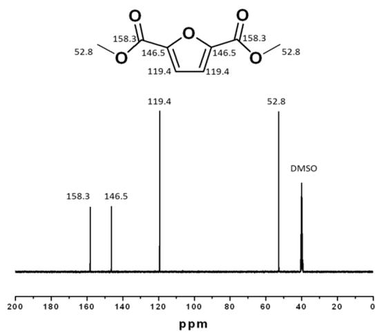
**Figure S2** <sup>13</sup>C-NMR spectra of dimethyl furan-2,5-dicarboxylate
