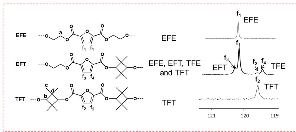
**Figure S3** Chemical structures of EFE, EFT, TFT and the peak assignment in  $^{13}\text{C}$ -NMR spectra
