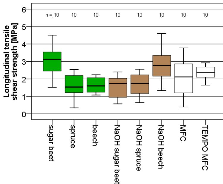
**Figure 6.** Box and whisker plot of the adhesive strength expressed by shear strength of bonded wood specimens for fibrillated material from different raw materials.
