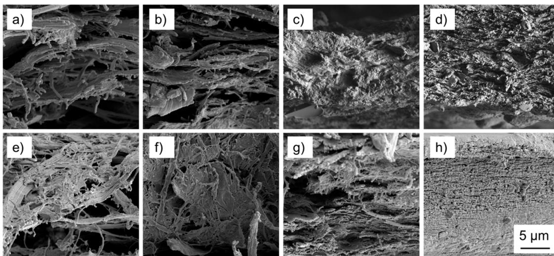
**Figure 5.** Representative SEM images of fracture surfaces of nanopapers after tensile testing: (a) spruce; (b) beech; (c) sugar beet; (d) MFC; (e) NaOH spruce; (f) NaOH beech; (g) NaOH sugar beet; (h) TEMPO MFC.
