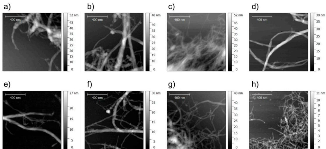
**Figure 2.** Atomic force microscopic (AFM) images of the smallest fibril fraction found in different fibril suspensions: (a) spruce; (b) beech; (c) sugar beet; (d) MFC; (e) NaOH spruce; (f) NaOH beech; (g) NaOH sugar beet; (h) TEMPO MFC.
