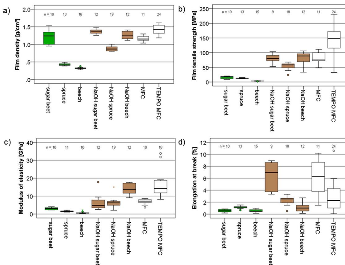
**Figure 4.** Box and whisker plots of (a) density; (b) tensile strength; (c) modulus of elasticity; and (d) elongation at break for nanopapers produced from different raw materials.
