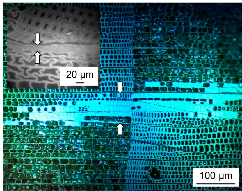
**Figure 7.** Incident light microscopic image of a typical wood adhesive bond line using the industrial wood adhesive urea-formaldehyde compared to a typical bond line using fibrillated material produced in the present study (inset). Arrows denote the approximate thickness of the bond line.
