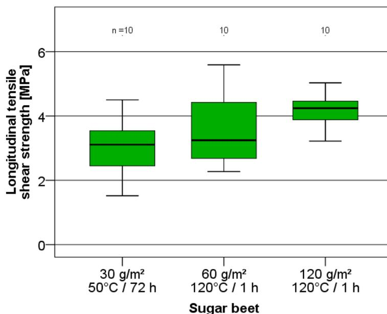
**Figure 9.** Box and whisker plot of the adhesive strength expressed by shear strength of wood specimens bonded with fibrillated sugar beet pulp using increasing spreading quantities.
