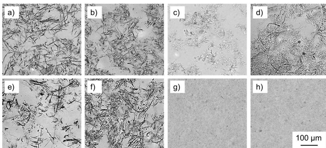
**Figure 1.** Light microscopic images of different fibril suspensions: (a) spruce; (b) beech; (c) sugar beet; (d) MFC; (e) NaOH spruce; (f) NaOH beech; (g) NaOH sugar beet; (h) TEMPO MFC.
