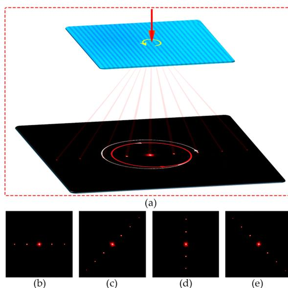
**Figure 5.** (a) Schematic diagram of the optical path for the beam steering characterization. (b–e) Diffraction patterns collected in the directions of  $0^\circ$ ,  $45^\circ$ ,  $90^\circ$ , and  $135^\circ$ , respectively.
