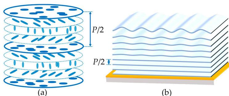
**Figure 1.** Schematics of (a) the cholesteric liquid crystal (CLC) helical structure and (b) the helical layers with a self-adapted distortion in a semi-free film. The distance between two adjacent layers equals to half a pitch. The orange layer represents the planar alignment film.
