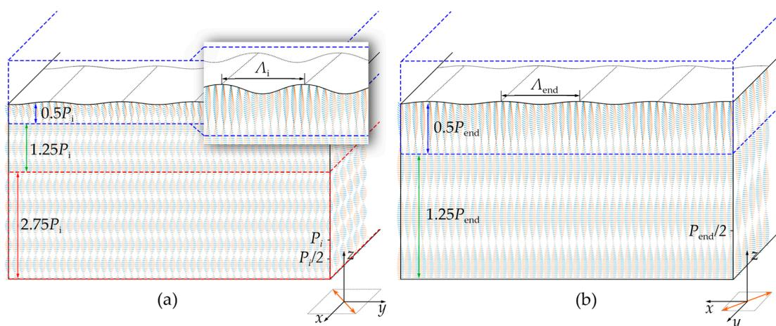
**Figure 4.** Simulated director configurations of the CLC grating (1 wt % ChAD-3c-S) at the (a) initial state and (b) end state. The inset in (a) shows a zoomed-in image. The anchoring directions are represented by orange arrows.
