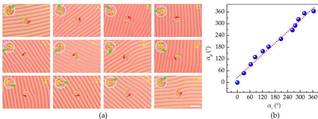
**Figure 6.** (a) Polarized optical microscope textures of the ZSM-5 zeolite microparticle rotation on the semi-free film. The enlarged microparticle is presented in the top left corner with a green dot denoting its orientation. The scale bar represents  $25 \mu\text{m}$  for all images. (b) Relationship between the rotational angle of the microparticle and that of the CLC grating. The dashed line is the linear fitting result.
