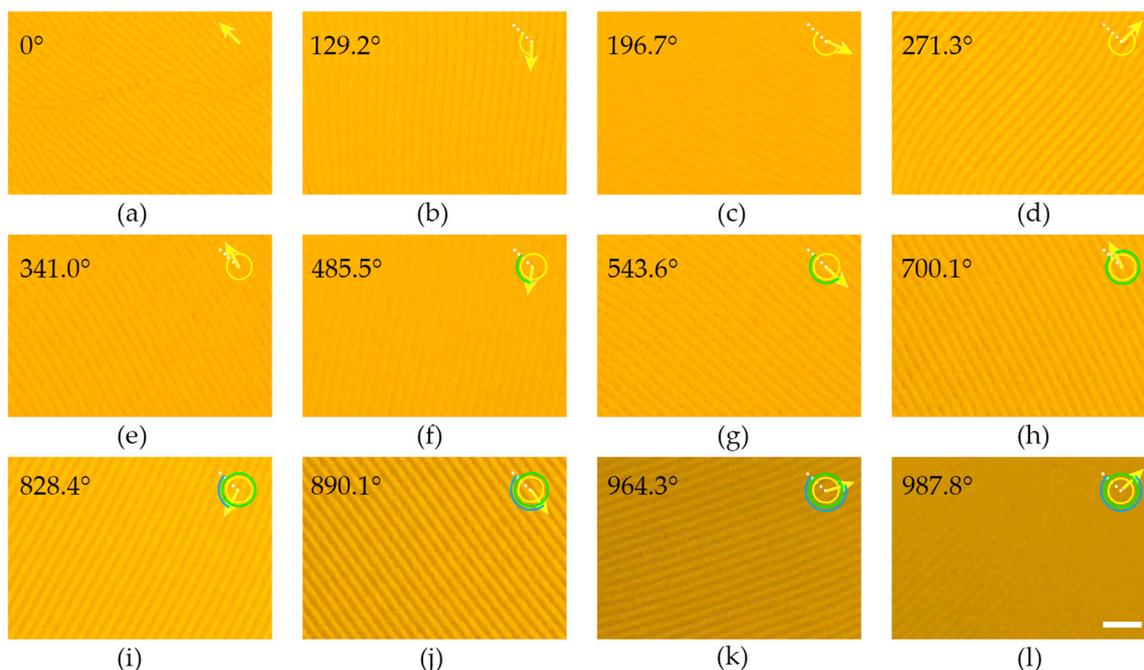
**Figure 2.** Light-driven rotation of the CLC grating (1 wt % ChAD-3c-S) along with the increasing exposure. The rotational angle is labeled in each top-left corner. The scale bar represents 25  $\mu\text{m}$  for all images.
