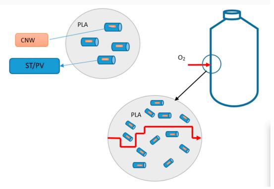
**Figure S1.** Schematical representation of the tortuous diffusion path generated by CNC containing fibers (PVST/CNC)f into PLA materials.
