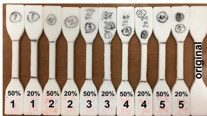
**Figure 9.** SPPM samples after heated at 50 °C for five minutes. In each sample, the applied programming strain is indicated at right above the hybrid type (1 to 5). The right sample is original as marked without any testing for comparison.
