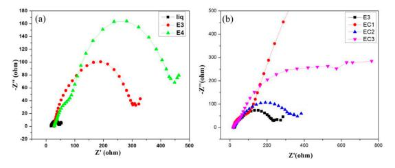
**Figure 10.** Nyquist plots from electrochemical impedance spectroscopy (EIS) showing the electron recombination resistance of DSSCs composed of (**a**) liquid electrolyte and gel electrolytes containing 1.4 g (E3) and 1.6 g (E4) of bare starch; (**b**) gel electrolytes E3, EC1, EC2, and EC3 containing 1.4 g bare starch and cross-linked starches A1, A2, and A3 respectively.
