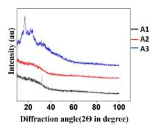
Figure 6. X-ray diffraction pattern of cross-linked starches A1, A2, and A3.
