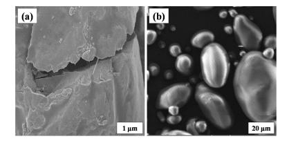
**Figure 8.** (a) SEM image of gel polymer electrolytes (E3) containing 1.4 g bare starch; and (b) granular structure of native starch.
