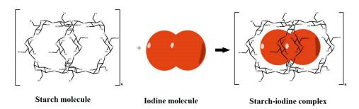
Figure 1. Schematic representation showing the formation of the starch-iodine complex.
