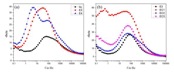
**Figure 11.** Bode phase plots of DSSCs composed of (**a**) liquid electrolyte and gel electrolytes containing 1.4 g (E3) and 1.6 g (E4) of bare starch; (**b**) gel electrolytes E3, EC1, EC2, and EC3 containing 1.4 g bare starch and cross-linked starches A1, A2, and A3 respectively.
