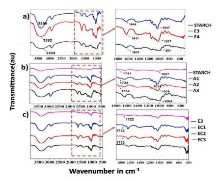
**Figure 5.** Infrared spectra of (**a**) native starch and gel polymer electrolyte containing 1.4 g (E3) and 1.6 g (E4) of bare starch; (**b**) native starch and cross-linked starches A1, A2, and A3; (**c**) electrolytes E3, EC1, EC2, EC3 prepared using bare starch and cross-linked starch A1, A2, and A3, respectively.
