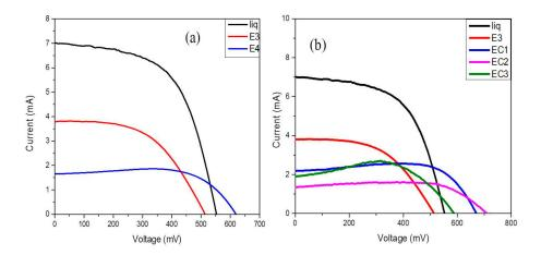
**Figure 9.** I–V curves of dye-sensitized solar cells (DSSCs) composed of (**a**) liquid electrolyte and gel electrolytes containing 1.4 g (E3) and 1.6 g (E4) of bare starch; (**b**) gel electrolytes E3, EC1, EC2, and EC3 containing 1.4 g bare starch and cross-linked starches A1, A2, and A3 respectively.
