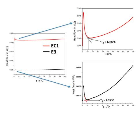
**Figure 7.** Differential scanning thermogram of an electrolyte containing bare starch (E3) electrolyte (EC1) containing cross-linked starch A1.
