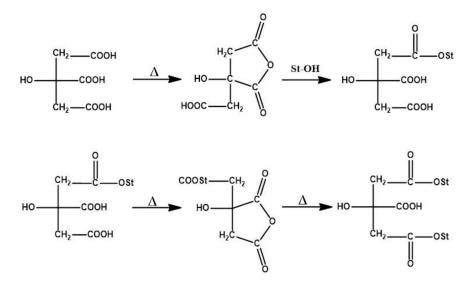
Figure 4. Mechanism of cross-linking of starch with citric acid.
