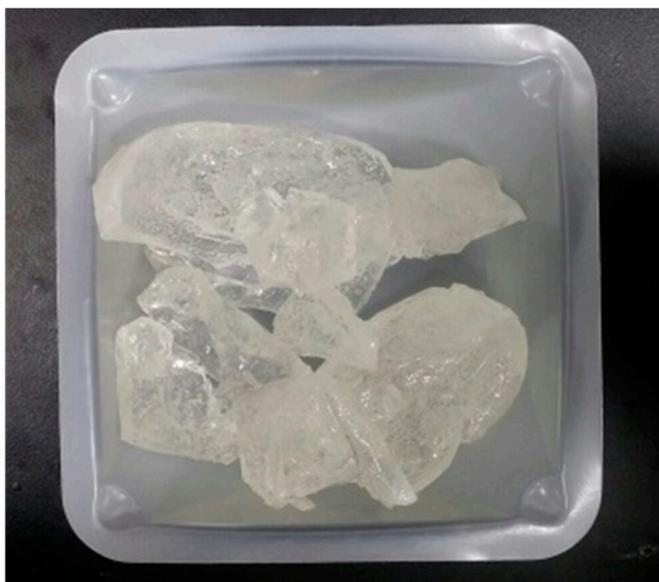
**Figure S3.** Photographs of cross-linked gels when macrodiols without the neutralization were used for the TPU synthesis.
