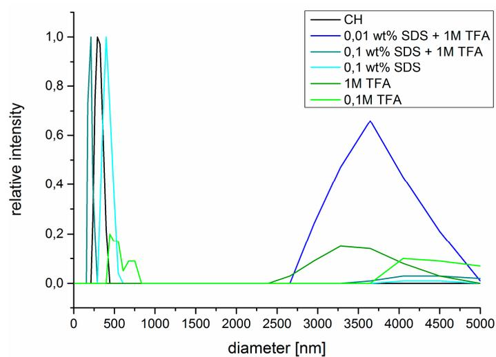
**Figure S5.** DLS results of the polyurea nanocapsules in cyclohexane and after redispersion into the different water mixtures.
