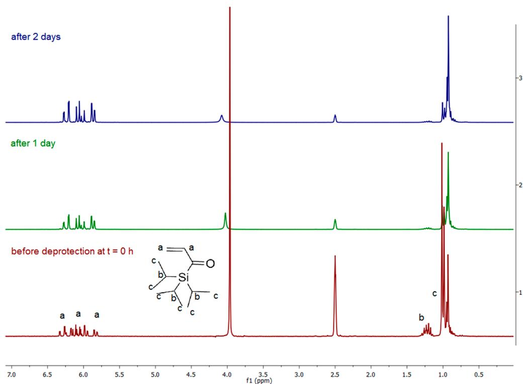
**Figure S8.** Kinetic measurements of deprotection of TIPSA with water measured by  $^1\text{H-NMR}$  spectroscopy in a solvent mixture of  $\text{DMSO-}d_6$  and  $\text{D}_2\text{O}$  (red:  $t = 0$  h, green:  $t = 1$  day, blue:  $t = 2$  days). The signal around 1.38–1.16 ppm completely disappeared and the signal at 1.03 shifted from the red to the blue and green spectra in 1.00–0.83 ppm region.
