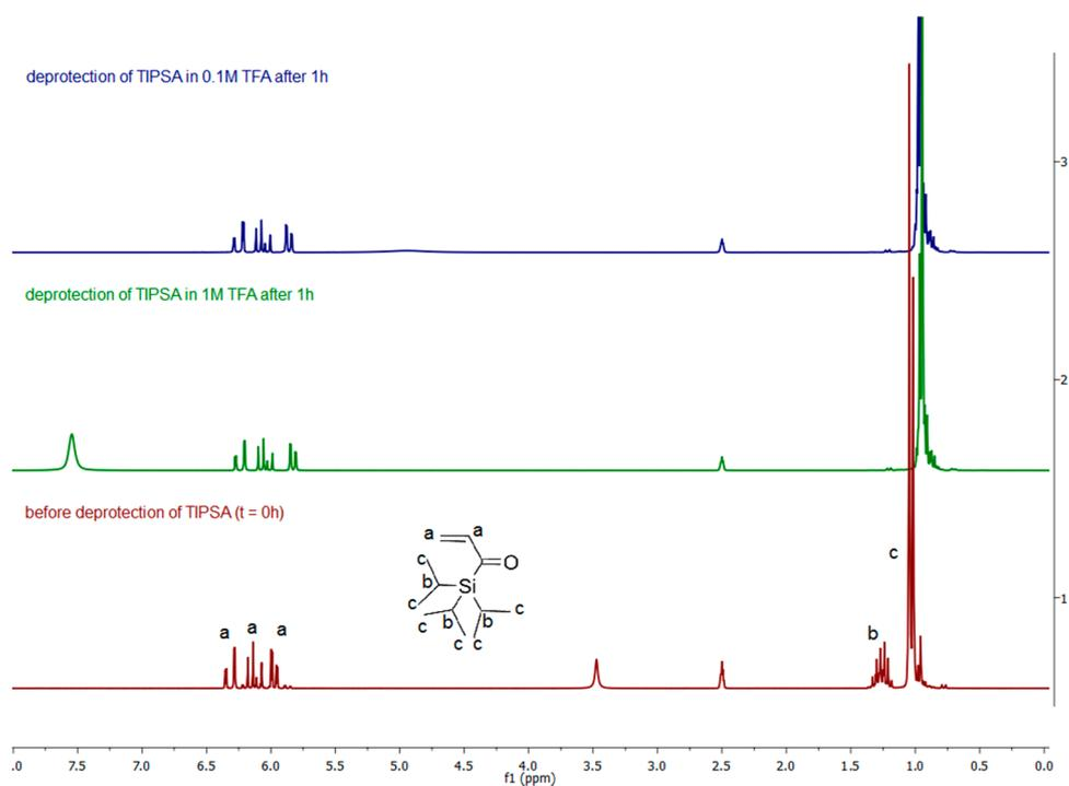
**Figure S7.** Kinetic measurements of deprotection of TIPSA using TFA measured by  $^1\text{H-NMR}$  spectroscopy in a solvent mixture of  $\text{DMSO-}d_6$  and  $\text{D}_2\text{O}$  (red:  $t = 0$  h, green: deprotection in 1M TFA at  $t = 1$  h, blue: deprotection in 0.1M TFA at  $t = 1$  h). The signal around 1.38–1.16 ppm completely disappeared and the signal at 1.03 shifted from the red to the blue and green spectra in 1.00–0.83 ppm region.
