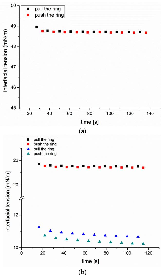
**Figure S4.** Interfacial tension measurement of cyclohexane and water ( $\sigma = 48.7$  mN/m at 22 °C) (a) and water-free formamide and cyclohexane ( $\sigma = 21.6$  mN/m at 22 °C) as well as water-free formamide and PTISPA-cyclohexane solution ( $\sigma = 10.3$  mN/m at 22 °C) (b).
