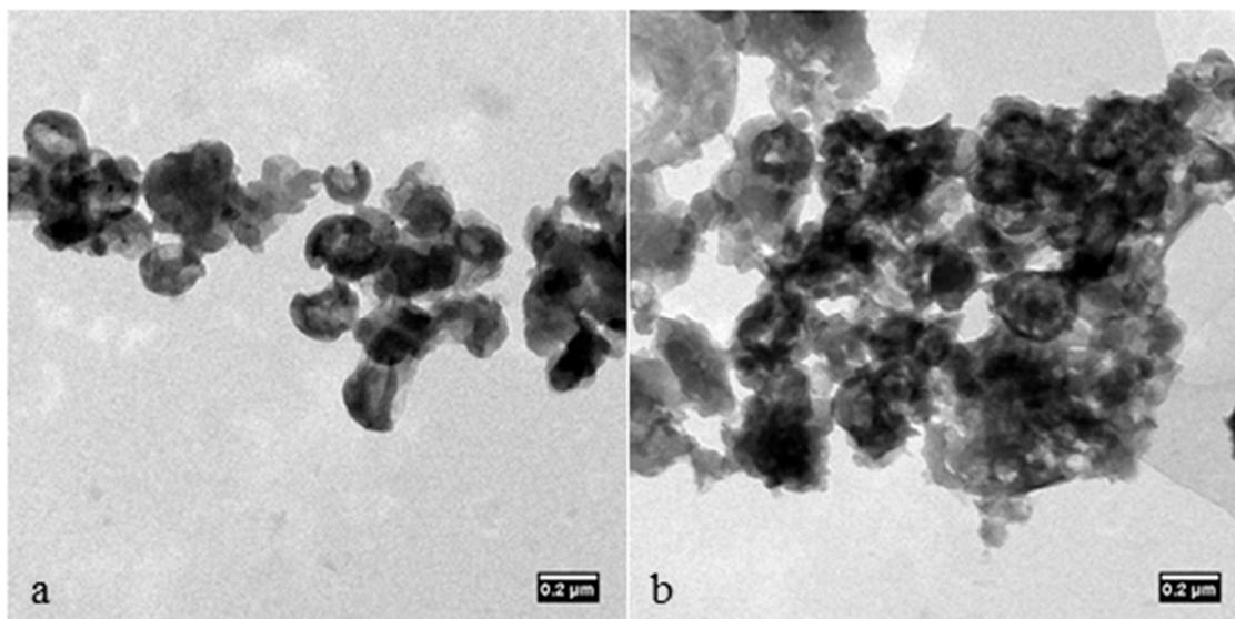
**Figure S6.** TEM images of polyurea nanocapsules in cyclohexane (a) and after redispersion in 0.1 wt % aqueous SDS solution (b).
