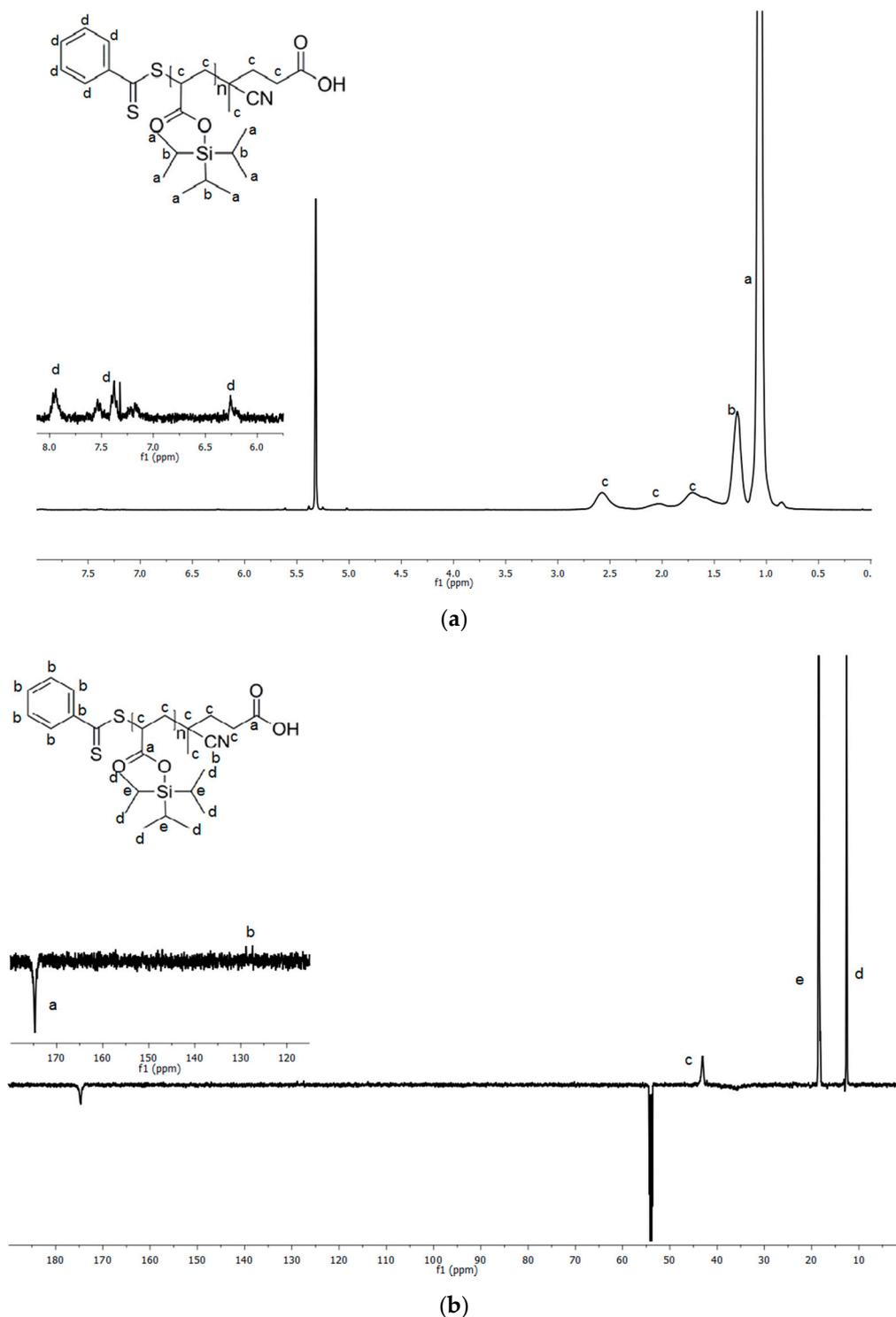
**Figure S1.**  $^1\text{H-NMR}$  (a) and  $^{13}\text{C-NMR}$  (b) spectra of poly(triisopropylsilyl acrylate) (PTIPSA) in deuterated dichloromethane.
