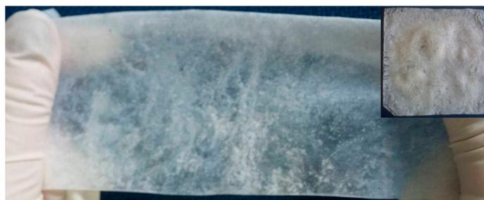
**Figure 4.** Membrane with P(ethylene-co-AAc28)/P(SSNa-co-GMA0.2)/PEG composition 60/10/30 after the total removal of the water soluble polymer (PEG).
