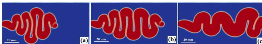
**Figure 3.** The buckling flow evolution varies with injection speeds of (a) 100 mm/s ( $t = 1.85$  s); (b) 200 mm/s ( $t = 1.35$  s); and (c) 300 mm/s ( $t = 0.95$  s).
