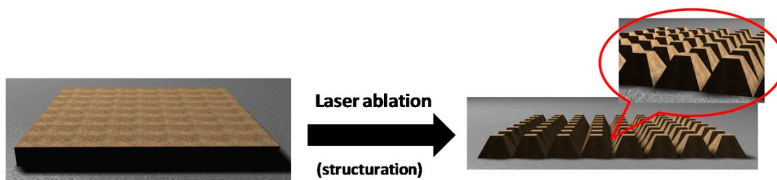
**Figure 2.** Structuration forming micropillars by laser ablation.
