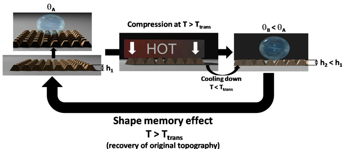
**Figure 1.** Schematic illustration of switching wettability from thermally induced surface shape memory recovery (from water contact angle  $\theta_A$  to  $\theta_B$  by compression, and recovery of the original  $\theta_A$  by heating).
