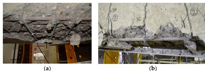
Figure 8. Separation of a large concrete cover in beam B60-214-1T-30 strengthened with 30 mm deep profile: (a) bottom side of beam with cut stirrups after T profile separation; (b) debonding of profile with concrete cover separation.
