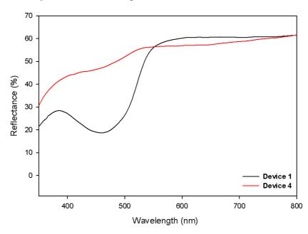
Figure 7. Reflection spectra of Device 1 and Device 4.
