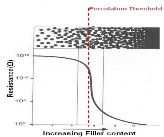
Figure 2. A sketch showing resistance decrease with sufficient filler connections.
