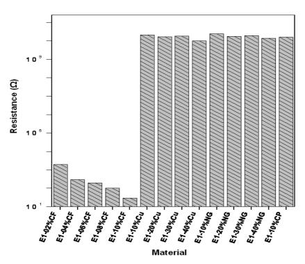
Figure 1. Resistance of E1 reinforced with conductive fillers.
