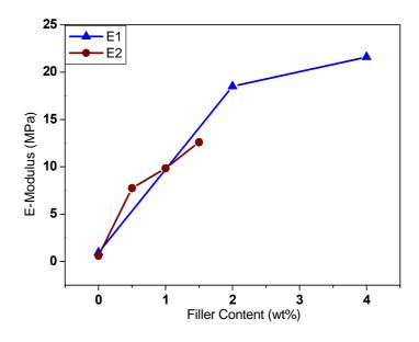
Figure 8. E-moduli for E1 and E2 with CF.
