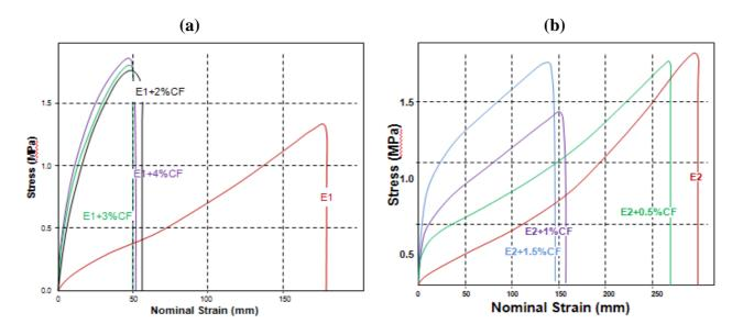
Modulus of elasticity or E-modulus is an indication of a material's stiffness and is determined by the slope of the stress-strain curves of the material [19]. The E-moduli for the compounds of E1 and E2 with carbon fibers are shown in Figure 8. The stiffness of the materials increases with the increasing filler concentration.
