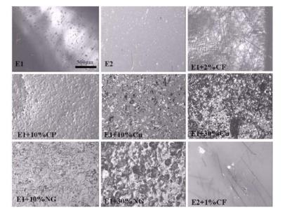
**Figure 4.** Optical microscopy of E1 and E2 filled with conductive fillers.
