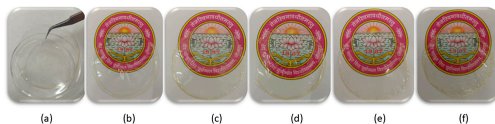
Figure 6. Digital images illustrating the transparency and opacity of the prepared films. (a) A representative thin film was placed on a petri dish without any background visualization. (b) CTS/Starch film (sample A). (c–f) CNP-CTS/Starch nanocomposite films with progressively increasing CNP loading (Samples B, C, D, and E, respectively). Images (b–f) are positioned over the logo of Veer Bahadur Singh Purvanchal University to visually demonstrate the films' decreasing transparency and increasing opacity with higher CNP content.
