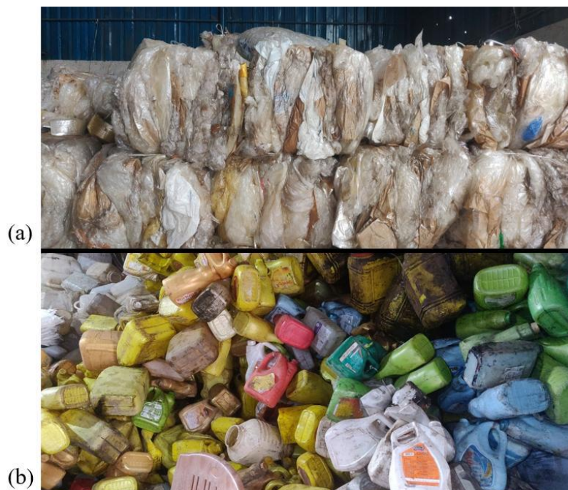
Figure 3. Segregation of plastic types (a) LDPE and (b) HDPE.
