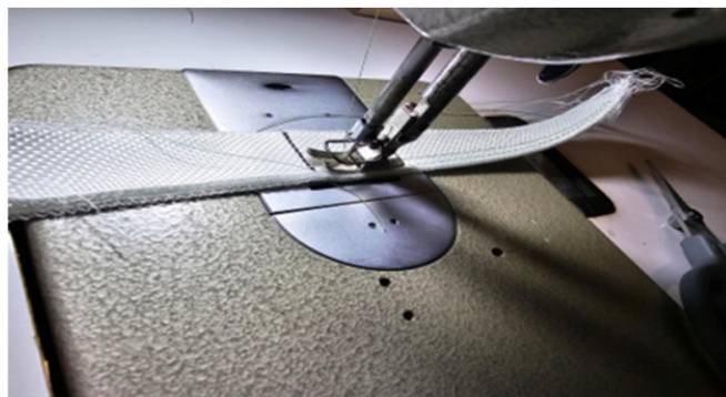
Figure 3. Stitching on Mercury MZ 20 43 sewing machine (DP \times 5 needle, 2 mm).
