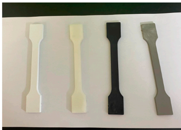
Figure 1. ISO 527-1 tensile test specimen geometry used for PA6, PA6 GF20, PA66, and PA66 GF20 materials.
