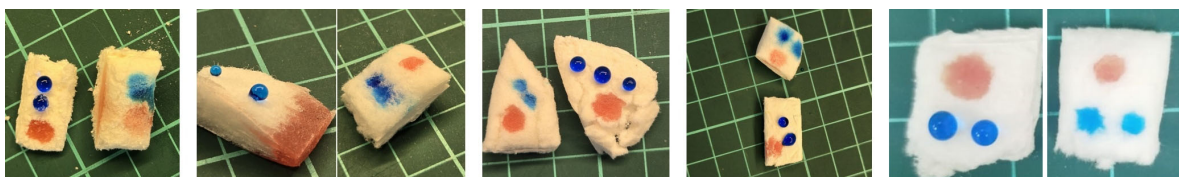
Figure 7. Comparative images of water (blue) and oil (red) droplets placed on CS and MCS sponges—left to right: samples derived from RH, CHS, TD, CP and CL.
