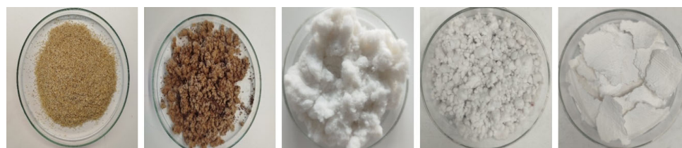
Figure 2. Ground raw materials used in the study (left to right): RH, CHS, CL, TD and CP.
