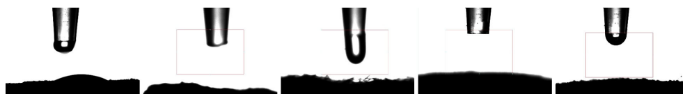
Figure 5. Images showing that water droplets placed on CS samples were instantly absorbed, leaving no measurable contact angle (left to right: CS-RH, CS-CHS, CS-CL, CS-TD, CS-CP).
