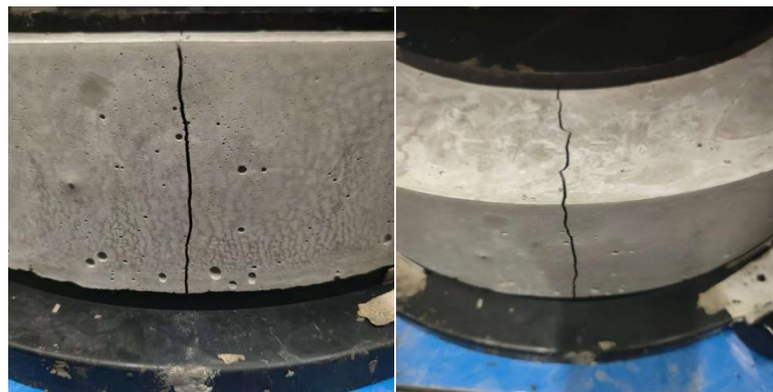
Figure 10. Cracking of the circular specimen.
